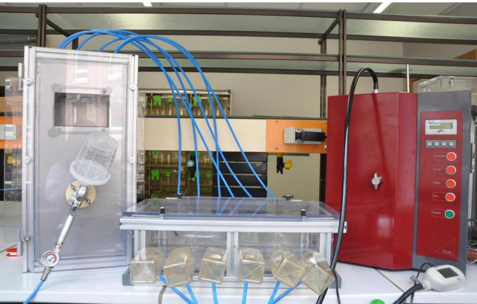
Inhalation model designed for in-vivo experiments on mice. The system is composed of a mixing chamber, an animal cage and ELPI instrument.
