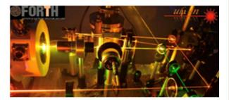
Laser patterning is a material independent technique for the controlled patterning of materials at the both the micro- and the nano- length scales. The technique offers the ability to directly write patterns on the surface as well as complex 3D channels into the bulk of solid materials, including biomaterials. Various
